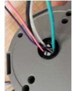
1. This fixture can be installed directly to a flat surface or as a pendant with a 1/2-inch conduit fitting. Splice connections can be made inside the fixture housing. To gain access to the fixture housing remove fixture back plate by removing the 4 #8 -32 stainless steel screws on the back plate
